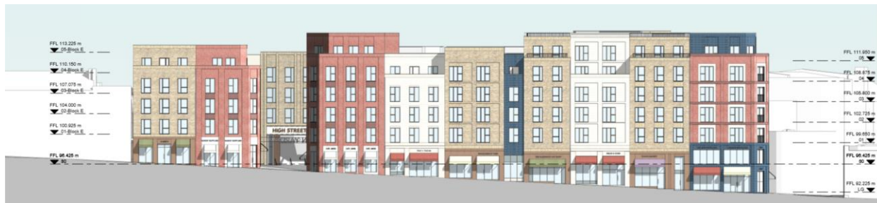
Figure 3: Union Street Elevation: demonstrating the vertical emphasis, individual units, and varying building heights.
