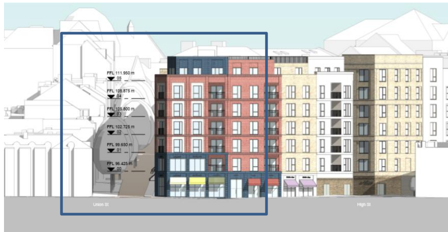
Figure 7: blue box demonstrating noise affected balconies
